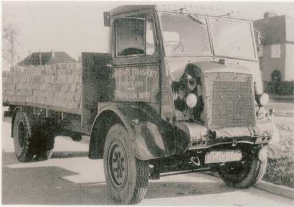
4-wheeler fitted with Perkins P6 engine and Albion Front axle
